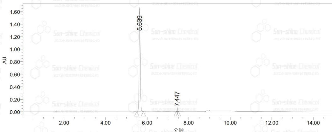
SampleName EX-527; Vial 1:b,7; Injection 1; Channel W2996 214.0nm-1.2; Date Acquired 2019-7-16 8:33:05 CST
